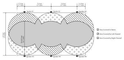
Figure 2 Stereo Coverage 6 speakers
